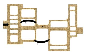
FIGURE 2 Critical Bottleneck in circuit. Pathway where the flow has to go from left to right (black arrow). \* Indicates the critical bottleneck. Bypass A will relieve flow obstruction, while B will have no effect on flow distal to the bottleneck. See the text for details
